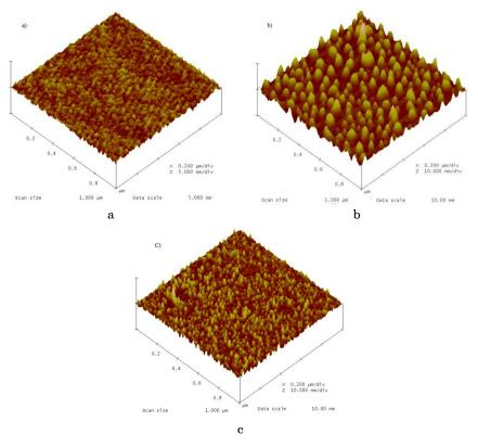
Fig. 1 – AFM images of bare c-Si waferas a reference (a), the 2 min 3 % HF etched c-Si wafer (b), 10 sec intrinsic a-Si:H layer deposited on c-Si at  $T_{Fil}=1500~^{\circ}\mathrm{C}$  (c)
